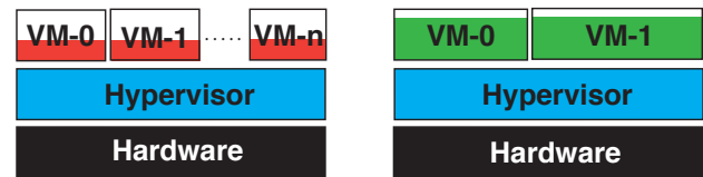
a) Server w/ Enterprise Workload b) Server w/ HPC-type Workload Fig. 1. Virtualized server illustration for a) enterprise workloads and b) HPC-type workloads.
